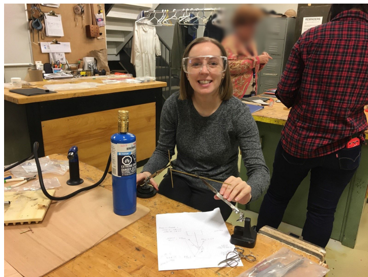
Preparing to solder a brass rod to hold a stone plumb bob
